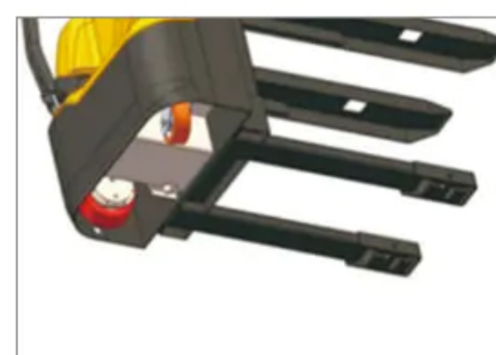
4 point design, improve the trucks stability.
