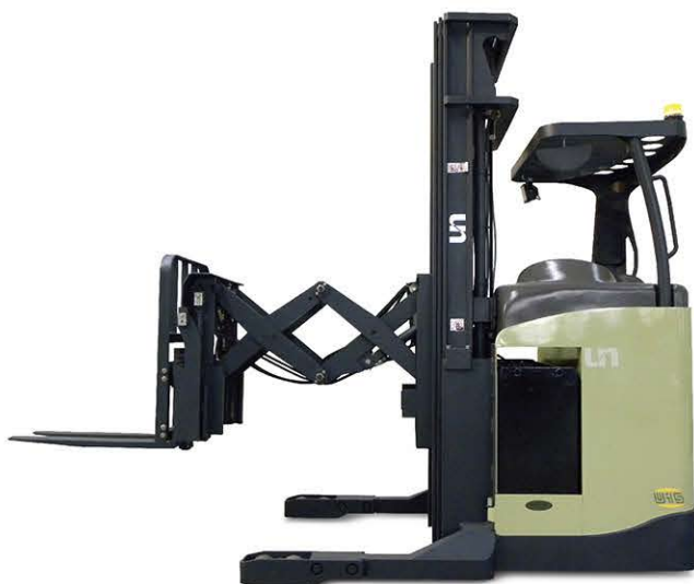
Double Deep Reach Truck capacity 1,500kg
